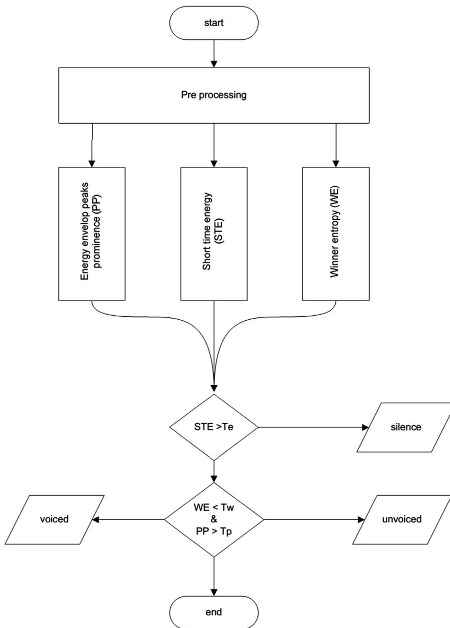
Fig. 2. Flowchart of the presented algorithm;  $T_e$ ,  $T_w$ ,  $T_p$  are threshold values for STE, WE and peak prominence, respectively, which should be adjusted according to the test condition and environmental noises.
