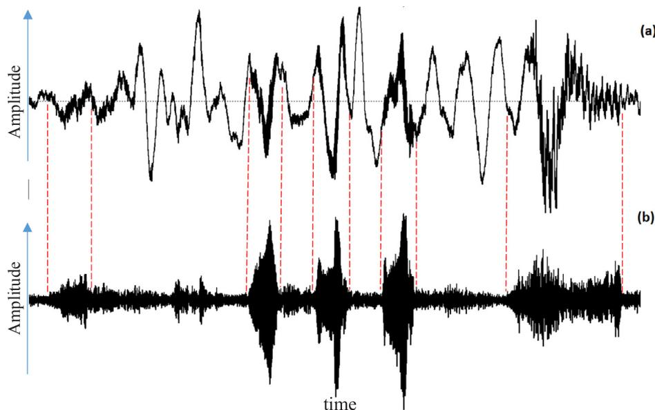
Fig. 1. (a) Raw signal recorded at a poultry house with noise; (b) filtered signal 'a' at chickens' vocal frequency range.
